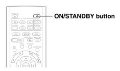
When the power turns on, ON/STANDBY indicator changes color from red (standby mode) to green (operation).
